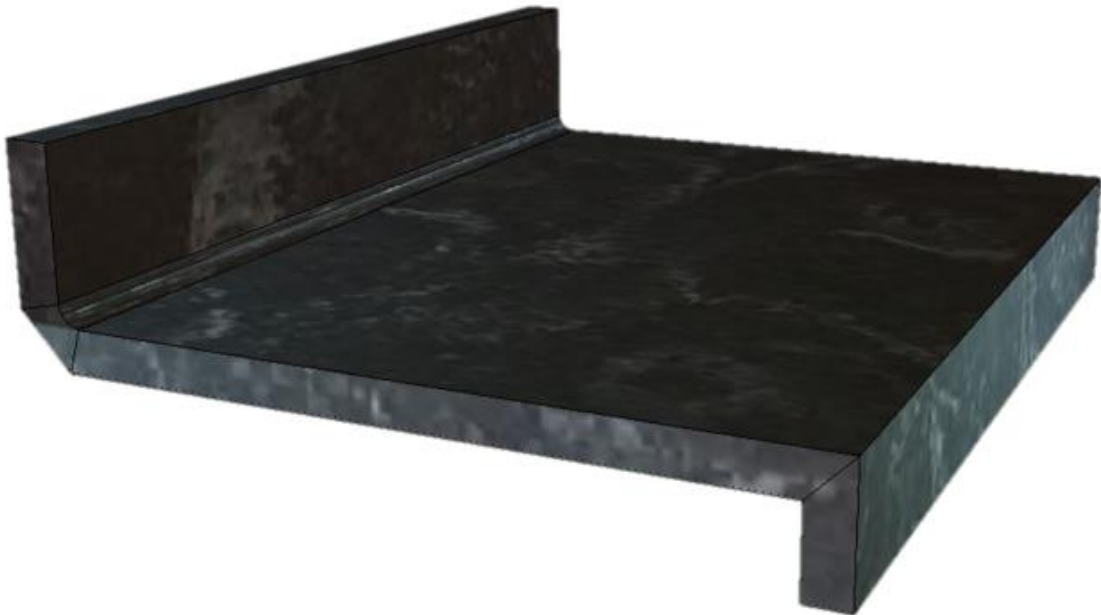
Figure 20. V-groove technique folded together
