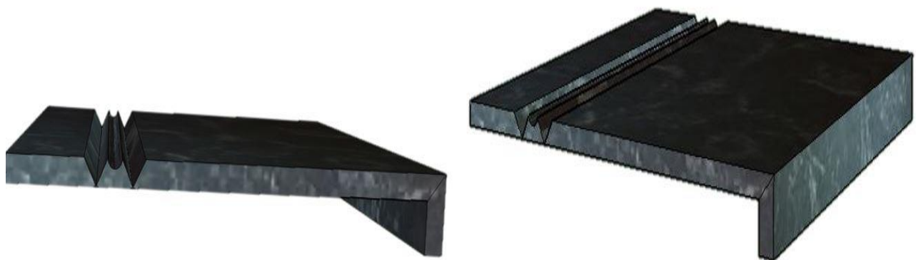
Figure 21. V-Groove edge before gluing and folding
