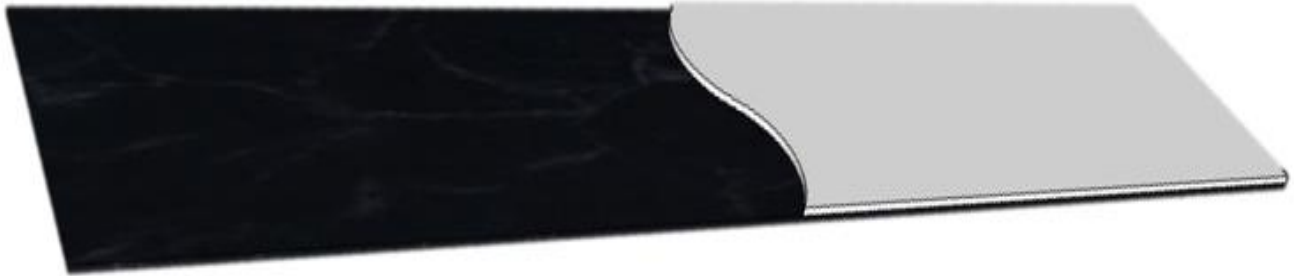
Figure 6. Template used to cut serpentine seam
